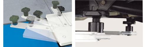
Swing board supporter equipped in upper lift can reach jacking point of SUV, VAN and so on.
