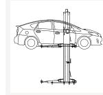
in the front side. Thus, width of lift is around 500mm narrower than the Symmetric type, which enables you to install the lift in a smaller space.
