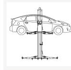
Long arms are used in all 4 arms. Thus, center of gravity of car stays near the center of the posts, which enables you to set up the vehicle from both directions.
